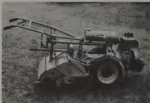
Howard Rotavator's largest walk-behind tractor, the "Gem," is shown above. It comes with either a 9.2 or 15.2 hp 4 cycle gas engine. With the smaller engine, this model costs $2,900. Dealers throughout the U.S.
